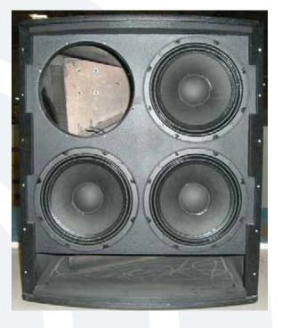
The picture above shows what the S410s looks like with the grill and top left woofer removed. Place the new woofer (part #0011737) where the old one was. Follow the same steps as above, but backwards 4 to 1. Power up the S410s and the new woofer should now be pumping out glorious lows. Awesome, you just replaced a 10" woofer!
